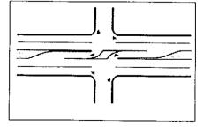
Figure 7B - 3-Leg Partial Access Median
