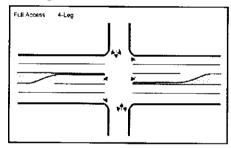
Figure 7C – Permitted Turns with Non-Traversable Median
