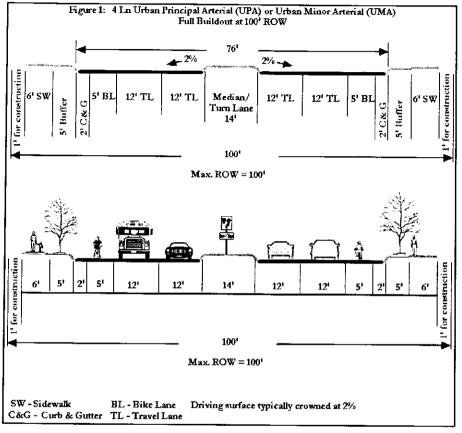
• Sidewalks are separated from travel lanes by a buffer strip.
