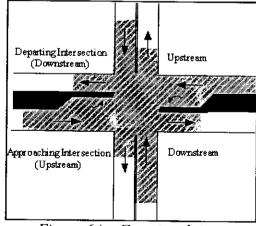
Figure 6A – Functional Area of an Intersection
