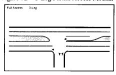
Figure 7D – Permitted Turns with a Two-Way Left Turn Lane (TWLTL)
