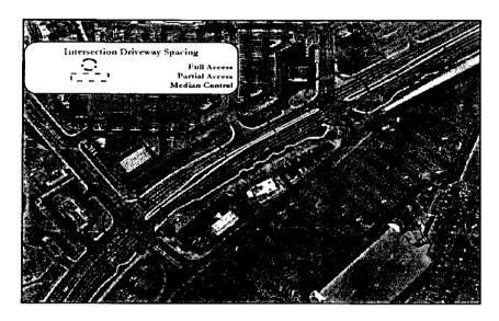
Beginning in 2008, NMDOT will reconstruct US 64 from Farmington to Bloomfield through several phases. Access management will be fully implemented through the corridor by means of consolidating driveways, improving median designs, building frontage roads, and adding signalized intersections.
