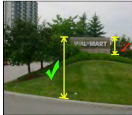
Area identified with the green check mark is the correct calculation for sign height (courtesy of the Signage Foundation).
