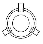
SET BASE ON SOLID CONCRETE BLOCK AFTER BACKFILLING PIPE
